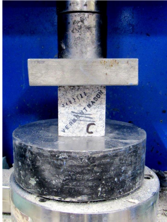
Sample during ASTM C 170 testing
