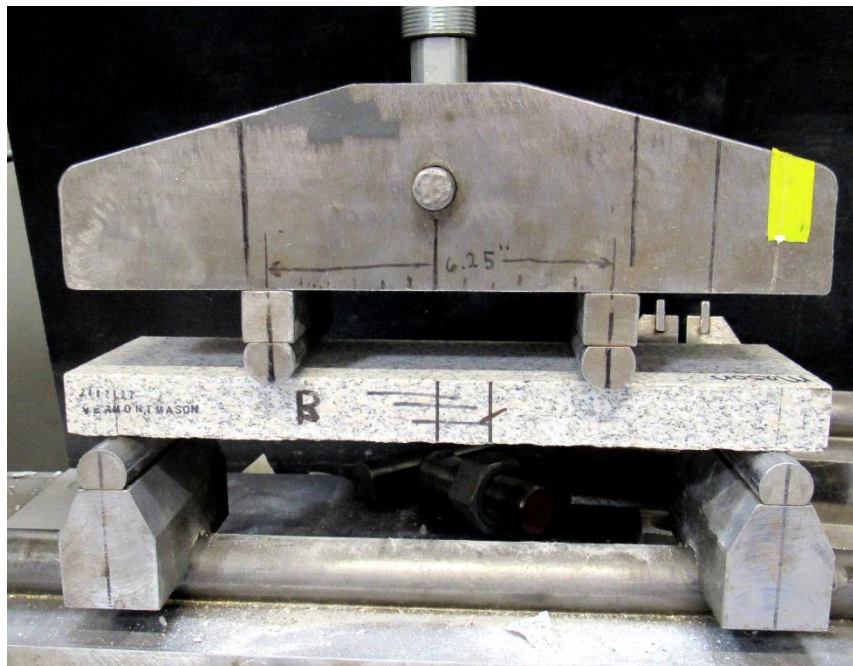
Picture of sample ready for ASTM C 880 testing
