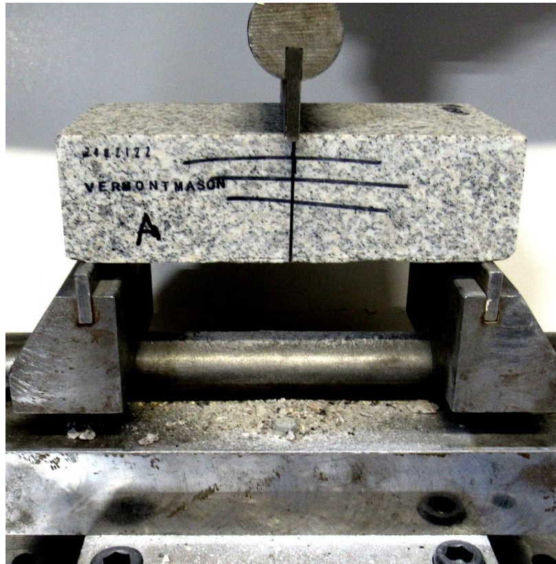
Sample during ASTM C 99 testing.
