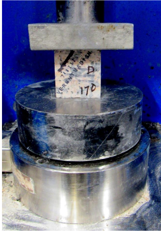
Sample during ASTM C 170 testing
