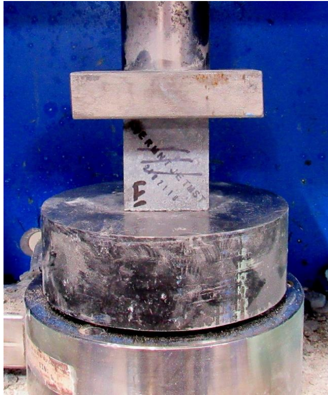
Sample during ASTM C 170 testing
